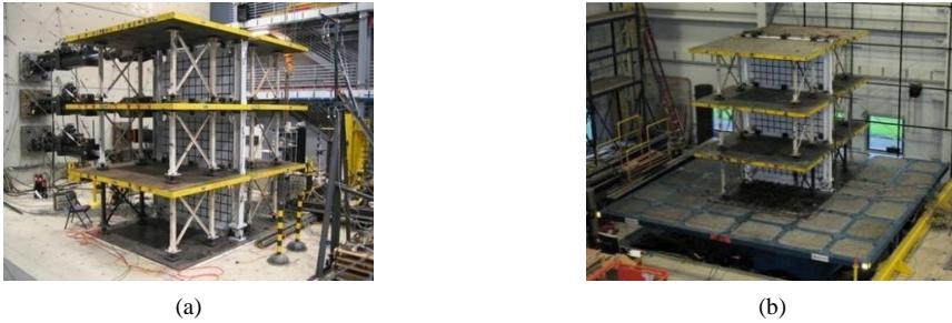
Figure 4. UB test set-up for (a) quasi-static and (b) shake table tests.
